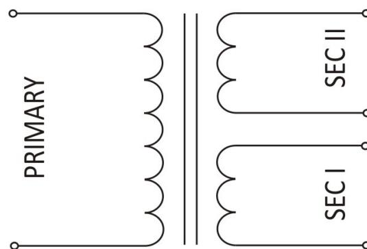
example, double secondary transformer – can be used series or parallel connected.
